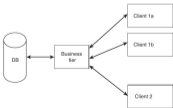
Figure 7.7 A three-tier style, in which clients do not connect directly to the database.
