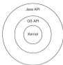
Figure 7.5 A common layered system, with the Java API implementation calling operating system functions, which in turn communicate with kernel functions.
