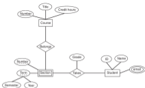
Figure 7.11 An entity-relationship diagram for courses, sections, and students in a course registration database.
