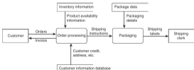
Figure 6.9 An example of a data flow diagram depicting a customer order system.
